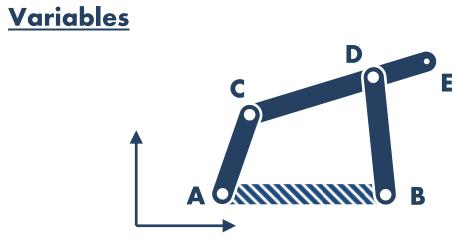
The linkage is fully determined by the coordinates of the fixed pivots A and B and the lengths of the links:
