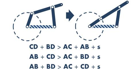
A small security constant s is added so that the lengths at the right are always at least a bit smaller than those at the left. Otherwise, the mechanism could collapse, in which case its behavior is undetermined.
