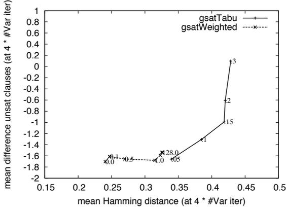
**Figure 11.** Diversification-bias plots of prohibition-based and penalty-based strategies (20:110 MAX-SAT instance). The curve named *gsatTabu* is labeled with the values for the fractional prohibition  $T_f$ , the curve named *gsatWeighted* is labeled with the  $\Delta w$  values for the weights update (points for  $\Delta w = 8, 16, 32, 64, 128$  are at a very similar position).
