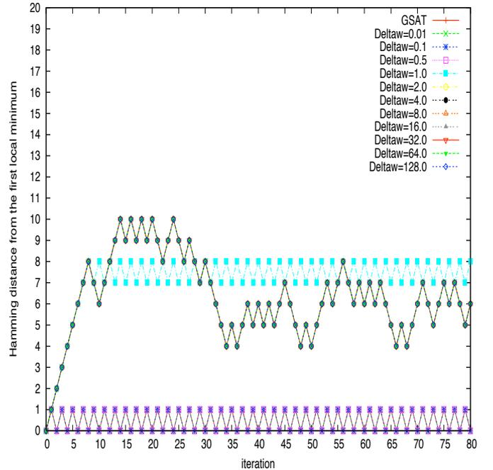
**Figure 14.** Evolution of the Hamming distance of single short trajectories of the penalty-based strategy. The curves for *GSAT* and  $\Delta w$  values smaller than 1.0 overlap (bottom of the Fig.), and the curves for  $\Delta w$  values bigger than 1.0 are the top ones overlapping.
