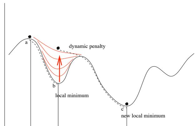
**Figure 1.** Transformation of the objective function to gently push the solution out of a given local minimum. Note: the intuition can be misleading for dynamically weighted clauses in MAX-SAT.
