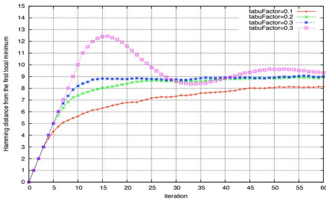
**Figure 15.** Performance of prohibition-based strategy during short trajectories. The values are averaged over 1000 trajectories starting at a different initial *FLM* point.
