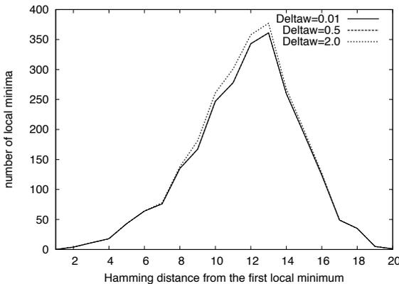
**Figure 8.** Distribution of the canceled local minima over different warped landscapes. The curves describe the landscape generated by a weight increase operation with different  $\Delta w$  values (0.01, 0.5, 2.0)
