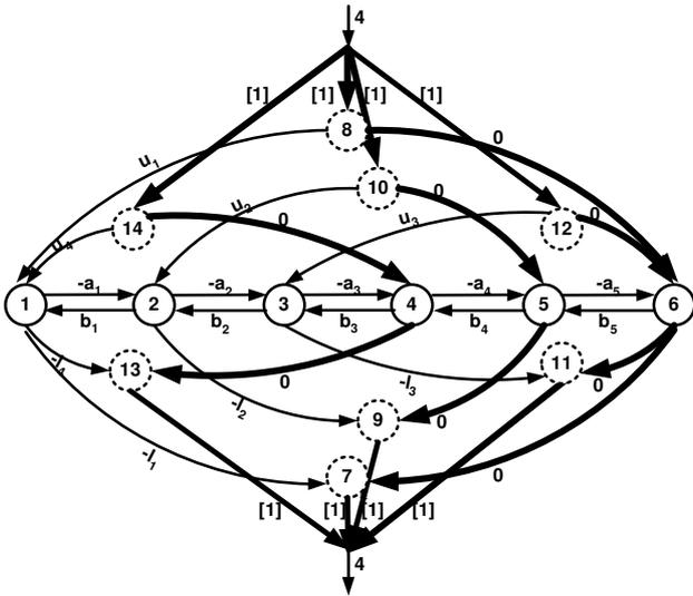
**Figure 4.** Network flow associated with the soft SLIDINGSUM constraint posted on the running example. The edge capacities are written in square brackets  $[]$  to differentiate them from the edge costs. Bold edges show a possible flow in the network.
