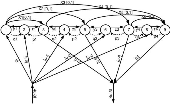
Figure 2. A flow graph for  $\text{SOFTSEQUENCE}(l, u, 3, t, [X_1, \dots, X_6])$
