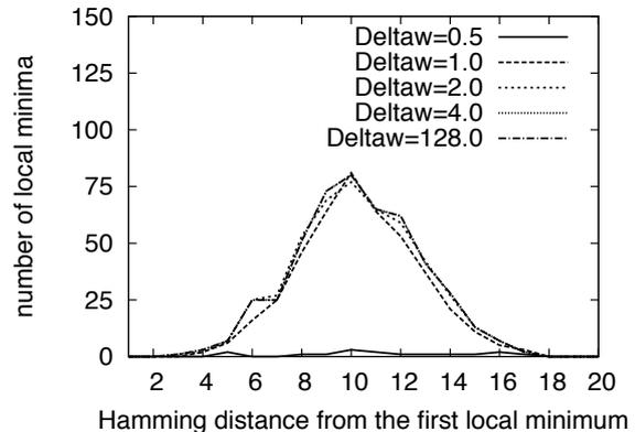
**Figure 2.** Distribution of the newly generated local minima over different warped landscapes. The curves describe the landscape generated by a weight increase operation with different  $\Delta w$  values (0.5, 1, 2, 4, 128). The curve for  $\Delta w = 0.5$  is at the bottom of the Fig.
