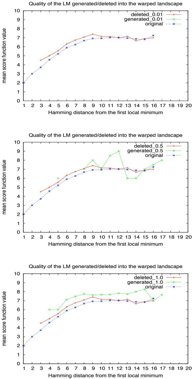
**Figure 5.** The mean quality of the generated/deleted local minima for the weight update values 0.01, 0.5, 1.0. The curve labeled as “original” shows the mean quality of the local minima in the initial fitness surface.
