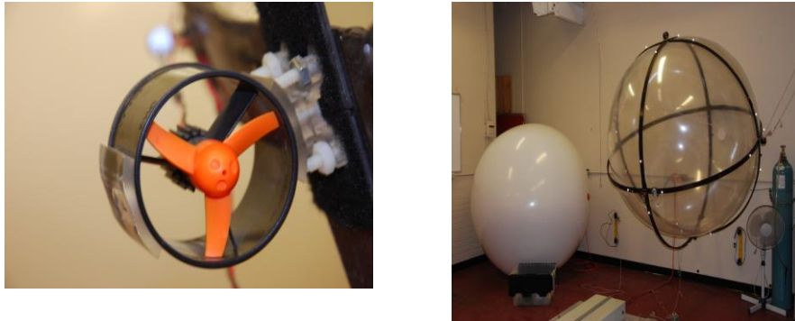
Fig. 3 Balloon propellers in the mount on the structure and Vicon marker cluster around one of the propellers
