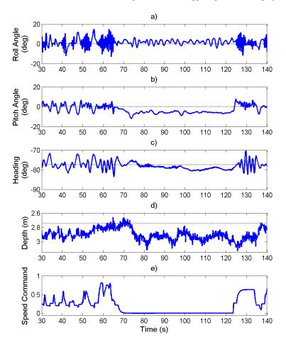
**Fig. 7** Performance of the autopilot system in hovering mode, with robot attitude a)-c) and depth d) over time, during one of the sea trials. The dotted lines in a)-d) correspond to the target values sent to the autopilot system. The open-loop speed command v in e) provided by the surprise module is unit-less: a value of 1.0 corresponded to maximum forward velocity of the vehicle.
