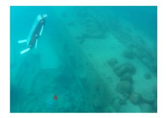
Fig. 1. The Aqua robot completes a vertical climb alongside a cargo vessel that rests on the ocean floor, prompted by a visual marker placed next to the ship by a human operator, seen near A. This is one of many new stable behaviors made possible by our technique. Image best viewed in color.
