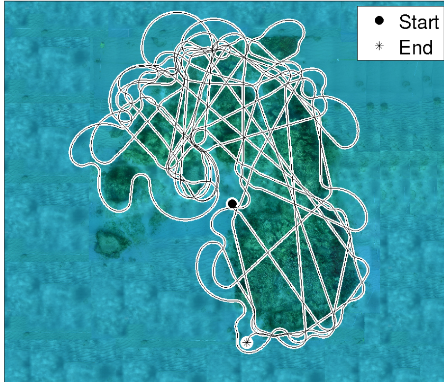
Figure 4. Path of the robot taken during one simulation run of 4000 iterations, overlaid over the coral reef image used to generate the simulated camera frames.
