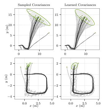
Fig. 5: Comparison of covariance estimations for *Wood Summer* (top) and *Gazebo Winter* (bottom). Every frame as 20 ICP odometry trajectories, although some are not visible because they are overlapping. The ground truth trajectory is shown as a thick black line. The green dots represent the final poses  $\hat{T}_F$ , while the green ellipses represent  $\hat{Y}_F$ . The data is projected on the ground plane for the sake of visualization.
